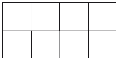
Fig. 3.14 The second order fundamental square edge net \langle 4 \rangle_2
